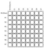
This is an example of how to draw and write the letter "A". Writes in binary according to: 0 = LED off 1 = LED on
